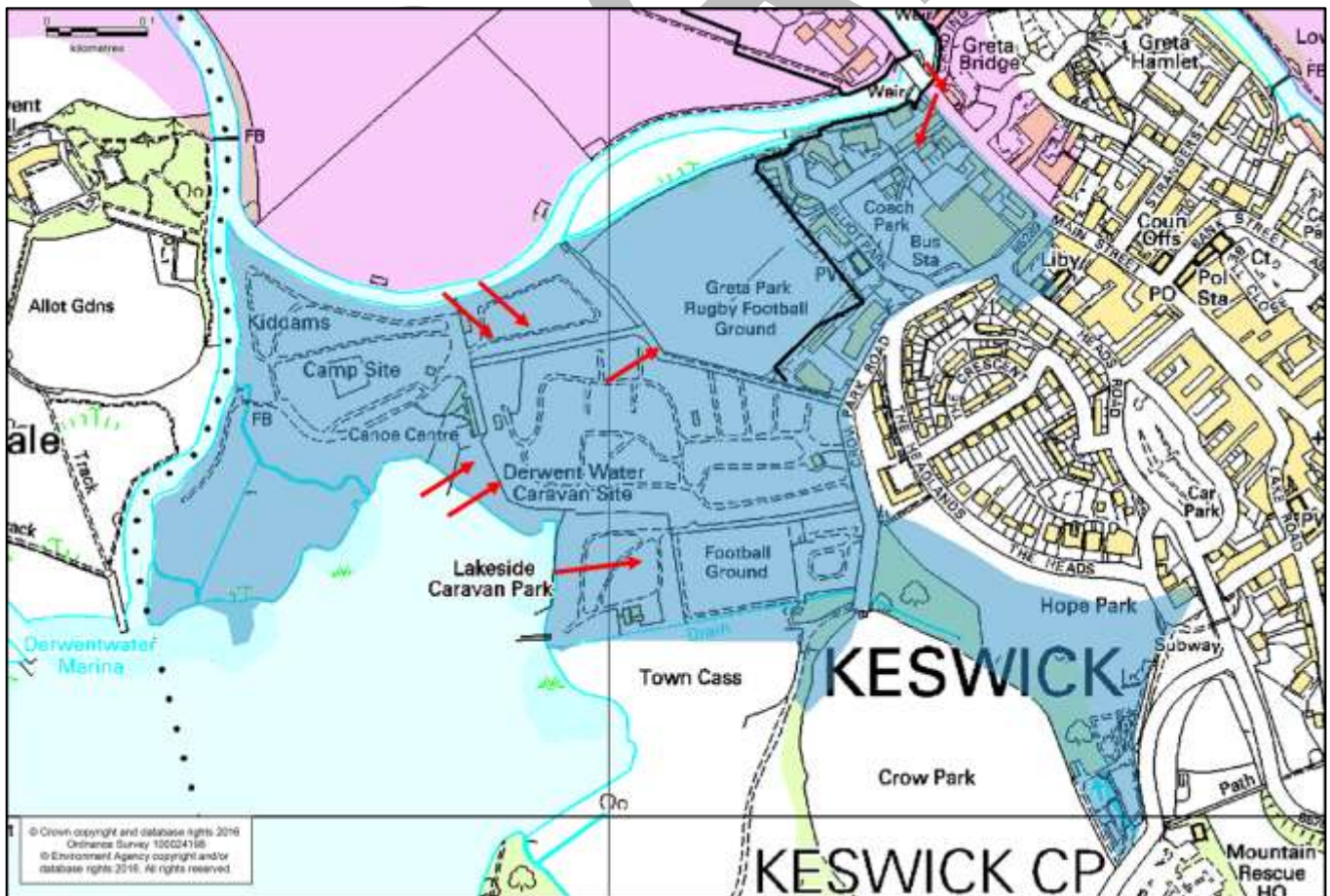
Figure 28 Source of Flooding and Flood Extent on the South of the Main Street
