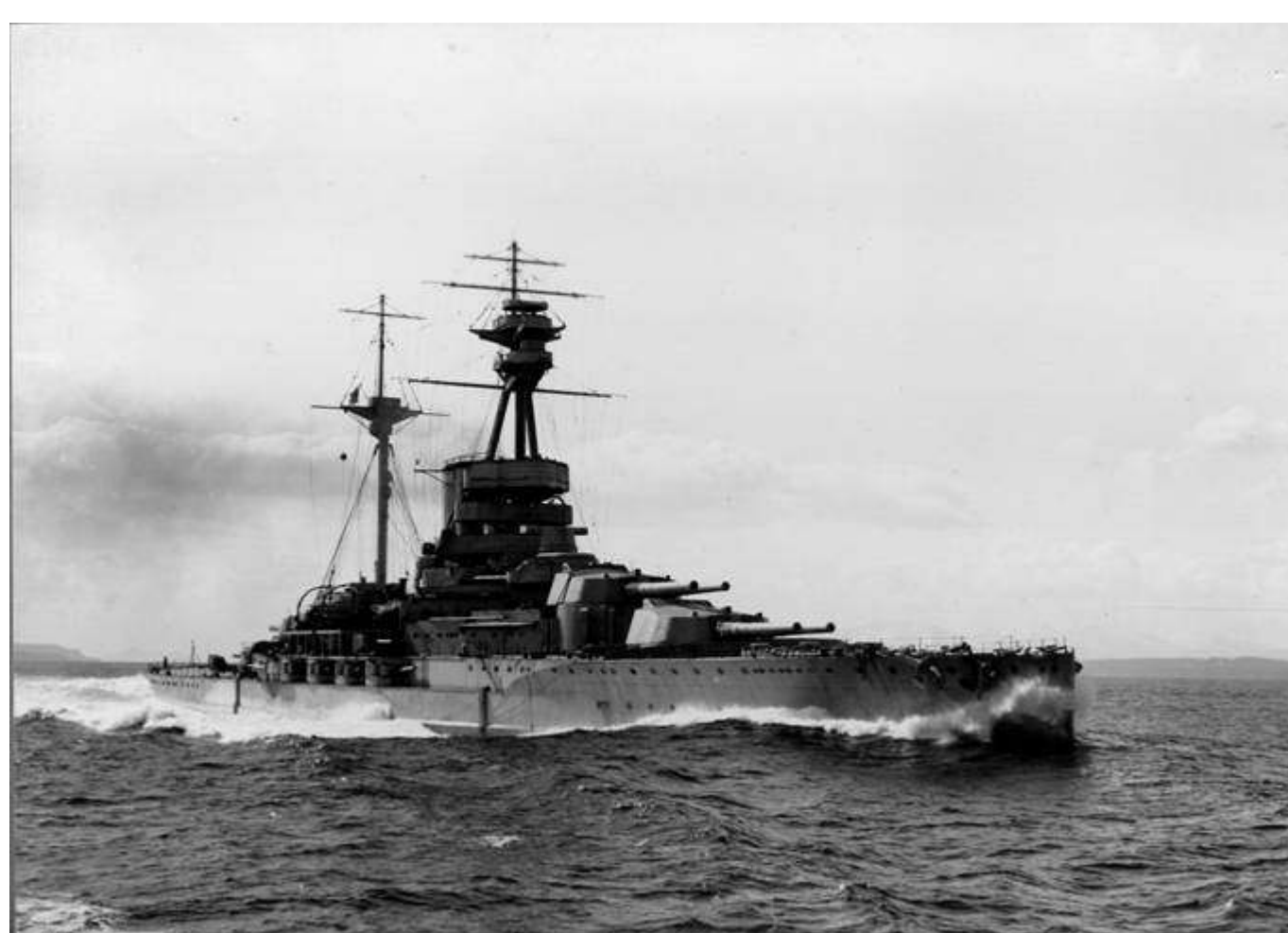
The battleship HMS Revenge which was built by Vickers in 1915. Vital statistics include: Length - 580 feet; Speed - 22 knots; HP - 42,600; Displacement - 28,000; Armament - 8 x 15", 14 x 6", 2 x 3"
