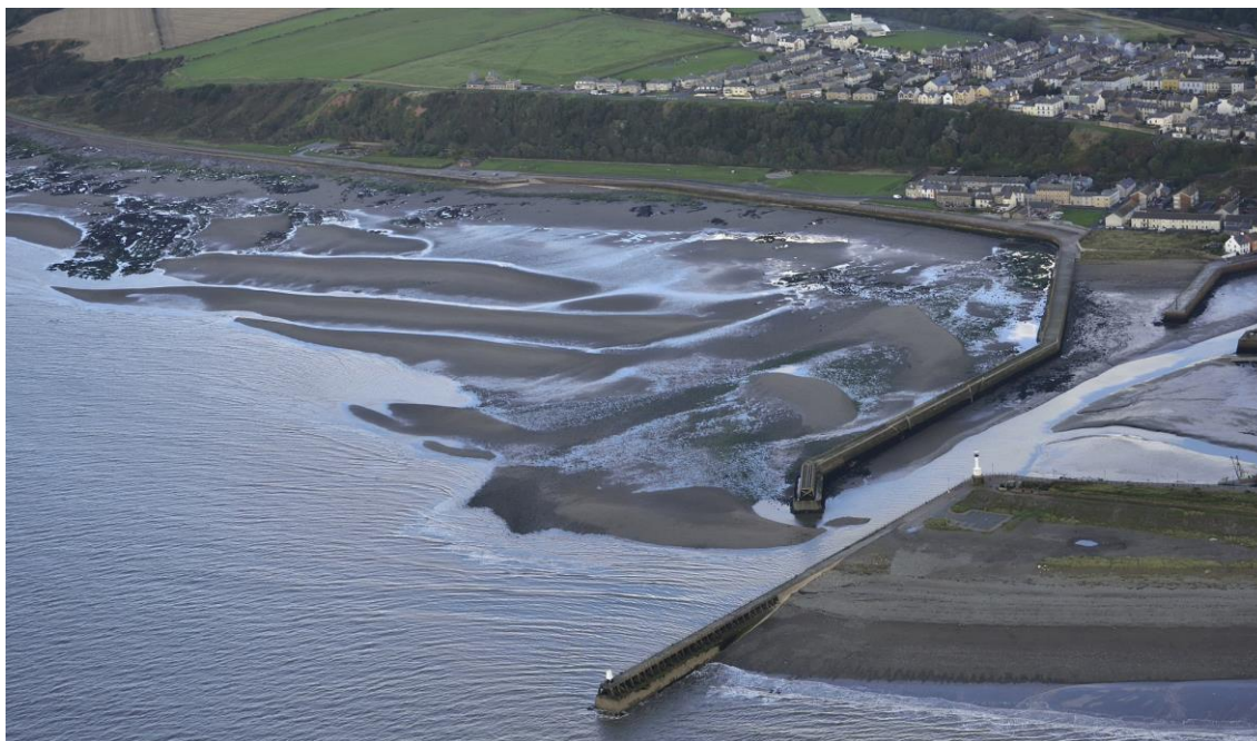
Figure 18 Unit 11e4.1 - showing the harbour structures and seawall, which fronts a low-lying hinterland backed by cliffs. Prior to construction of defences in 1930s there had been large scale erosion of these cliffs. The beach is characterised by mainly sand, with outcrops of sandstone exposed in places. Photograph ©North West Regional Monitoring Programme.
