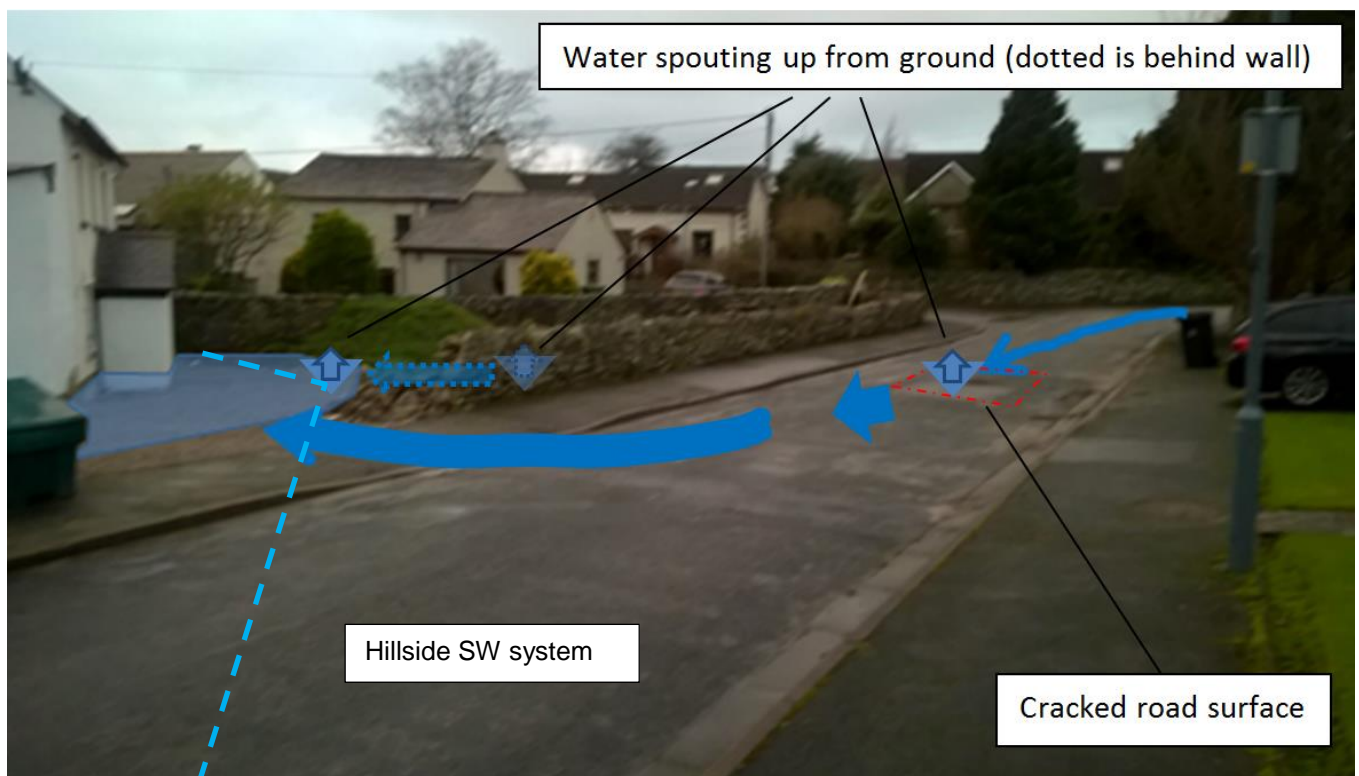
Figure 10: Flow routes around Springfield. Approximate line of culvert shown by dashed line.
