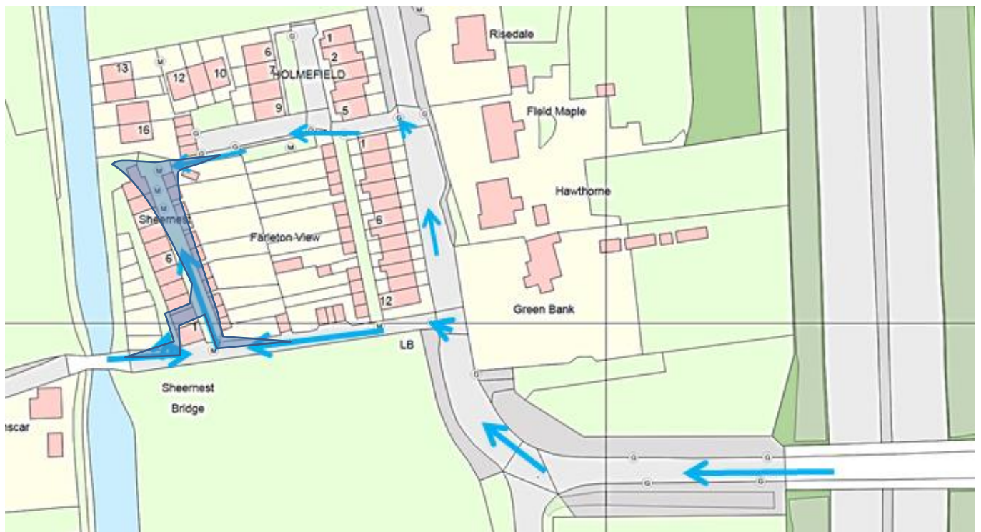
Figure 15: Extent of flooding and reported flows leading to Sheernest Cottages indicated by blue arrows.
