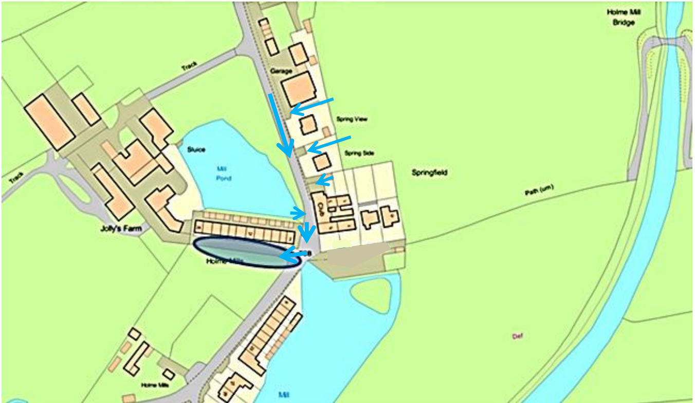
Figure 23: Flooding and flow routes at Holme Mills.
