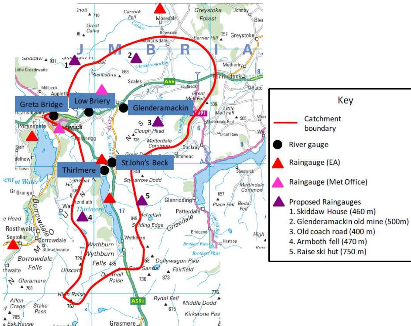
Figure 1: Approximate catchment of the River Greta upstream from Keswick, river gauges and existing and proposed raingauges within the catchment.
