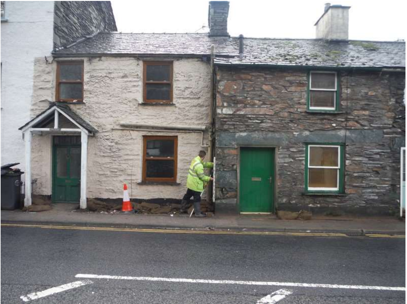
Figure 15 - Recorded water level at row of cottages on Rydal Road, situated opposite the Greenbank Ghyll culvert inlet shown in Figure 14
