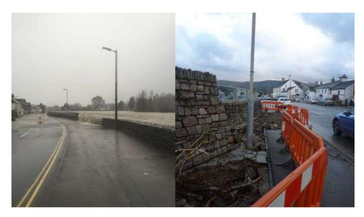
Photograph 25 and 26: Flooding at High Hill Road - Floodwall first overtopped where glass panels finish (left) and scoured footpath (right)
